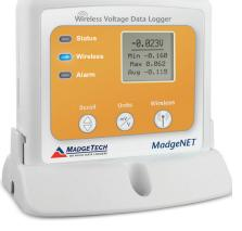
software. The statistics can be reset through the keypad of the device, allowing customers to keep track of statistics over certain time periods. This feature does not erase the data recorded, but only resets the statistics count.
