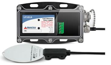
present. This low cost system comes complete with a data logger, weatherproof enclosure and leaf wetness sensor.
