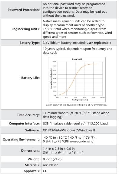
BATTERY WARNING: FIRE, EXPLOSION, AND SEVERE BURN HAZARD. DO NOT SHORT CIRCUIT, CHARGE, FORCE OVER DISCHARGE, DISASSEMBLE, CRUSH, PENETRATE OR INCINERATE. BATTERY MAY LEAK OR EXPLODE IF HEATED ABOVE 80 °C (176 °F).
